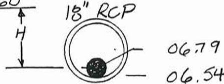
As a result, discharge from Pond B is throttled down to a rate of 2.07 cfs through the 18" RCP. This will discharge into the catch basin for pond A. The catch basin will have two chambers; one acting as a by-pass for Basin B and one throttling flow for Basin A.
