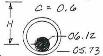
This will regulate the discharge into the ponding area below and east of the parking area, prior to discharge into the Corrales Acequia. Resultant inv. elev. 5.37
