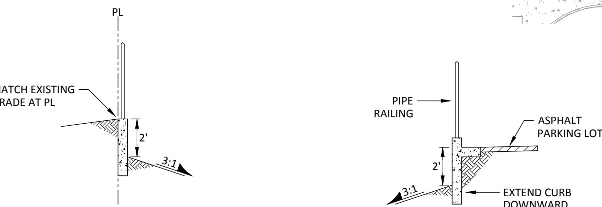
TYPE "A" CURB W/PIPE RAIL DETAIL NTS
