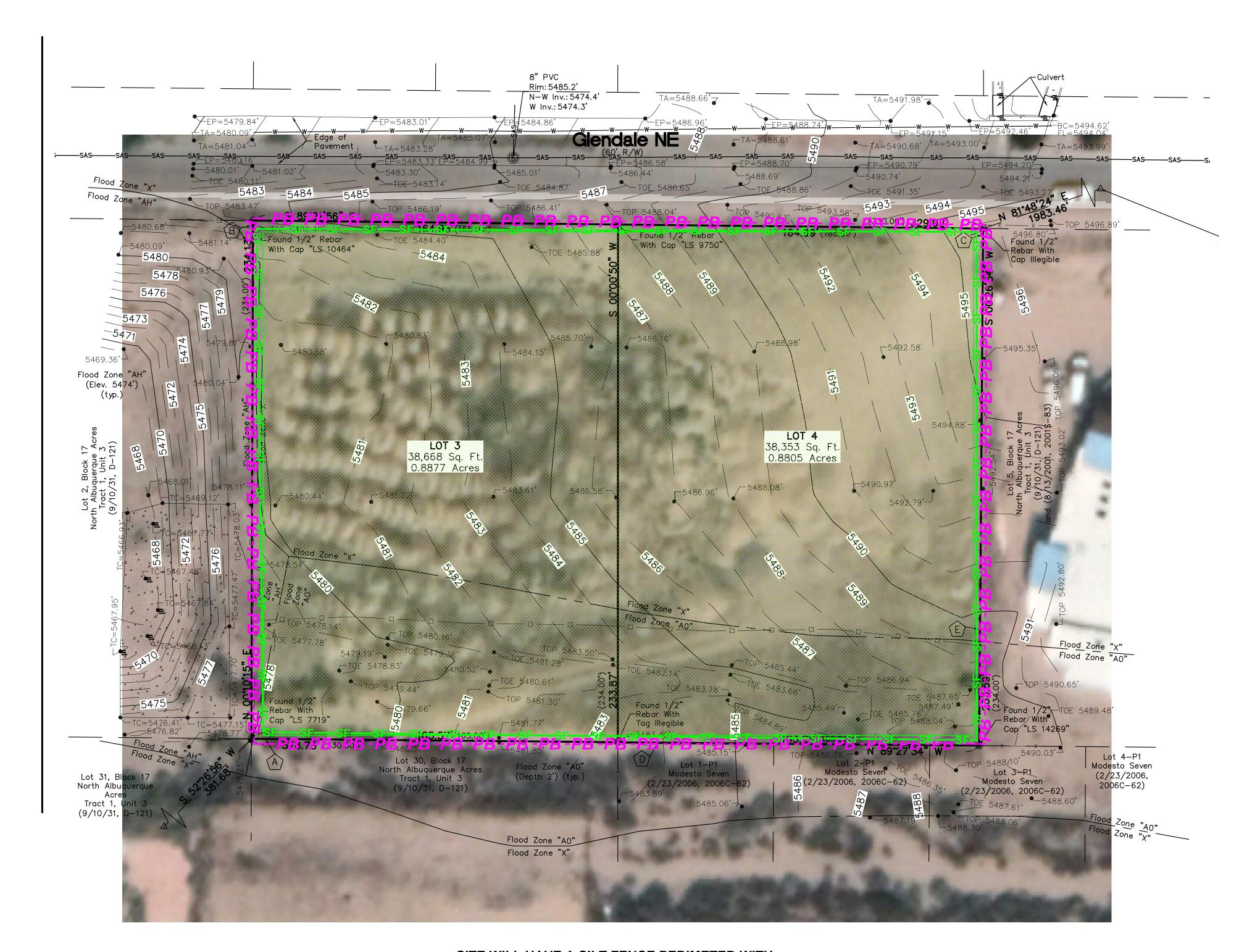
SITE WILL HAVE A SILT FENCE PERIMETER WITH HYDROSEEDING AND TACKIFIER
