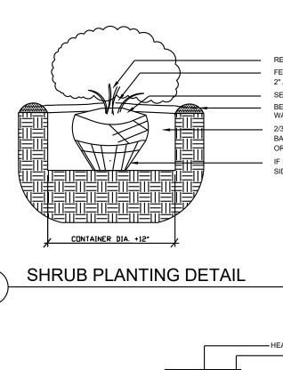
REMOVE PLANT IDENTIFICATION TAGS BEFORE JOB IS COMPLETE FEATHER MULCH TO A 2" DEPTH OVER PLANT ROOTBALL, KEEP MULCH 2" AWAY FROM CENTER OF SHRUB. NO WEED BARRIER OVER ROOTBALL. SET SHRUB ON UNDISTURBED PIT BOTTOM PLUMB AND STRAIGHT BERM REMOVED SOIL AT EDGE OF PLANTING PIT TO AID IN WATER RETENTION OVER ROOTBALL
