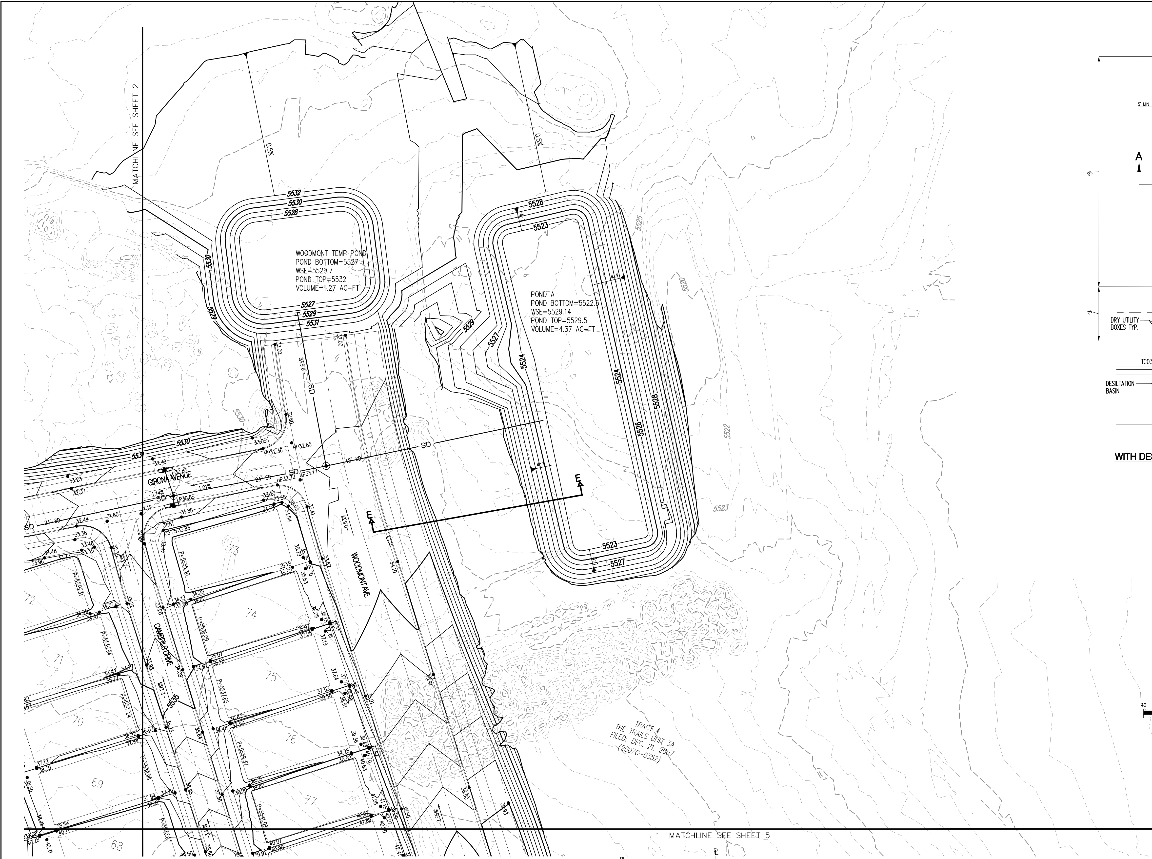
TYPICAL LOT GRADE DETAIL WITH DESILTATION BASIN FOR SEDIMENTATION CONTROL NOT TO SCALE
