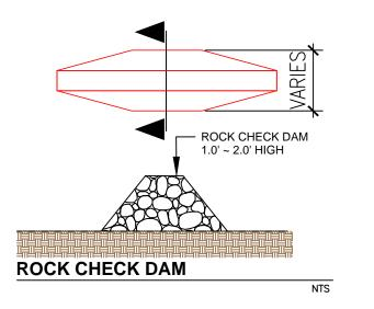
PLACE CHECK DAMS AT REGULARLY SPACED INTERVALS ALONG SWALE OR DRAINAGE DITCH.
