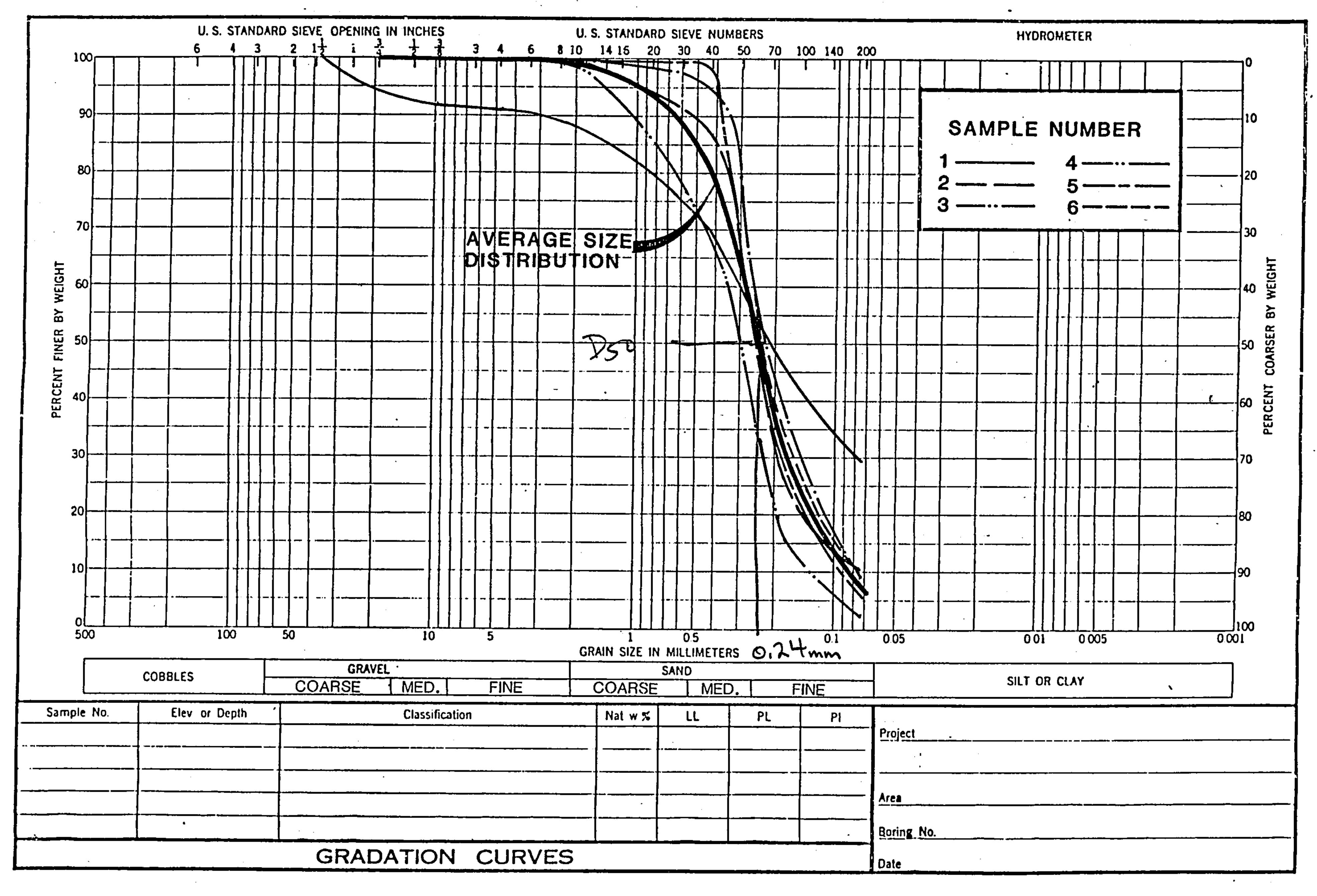
Figure 2.4. Sediment size distribution curves of surficial soil samples (see Figure 3.3 for sample locations).
