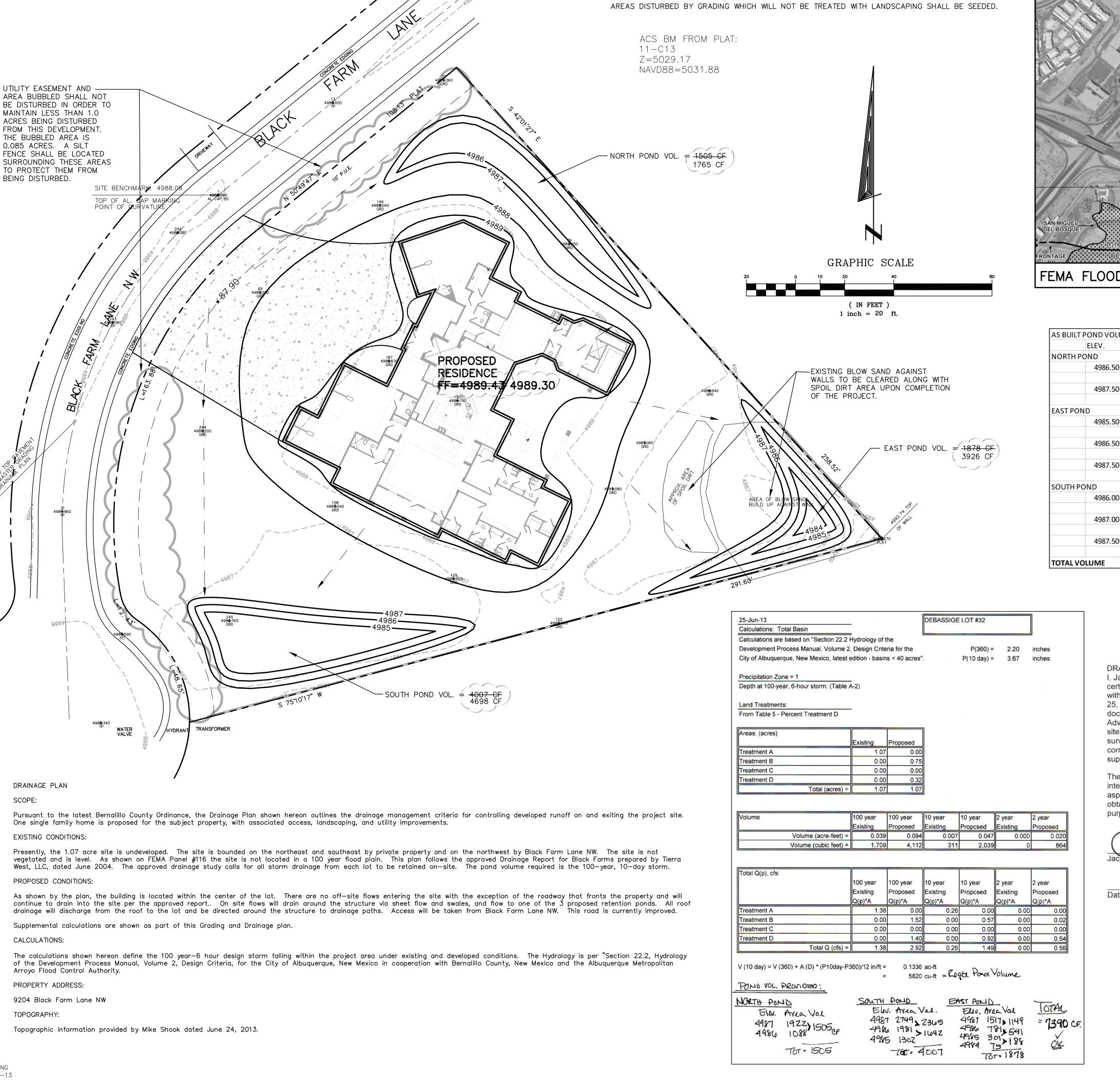
STANDARD GRADING NOTE: THE MAXIMUM GRADED SIDE SLOPE SHALL NOT EXCEED 3 FEET (HORIZONTALLY) TO 1 FOOT (VERTICALLY).
