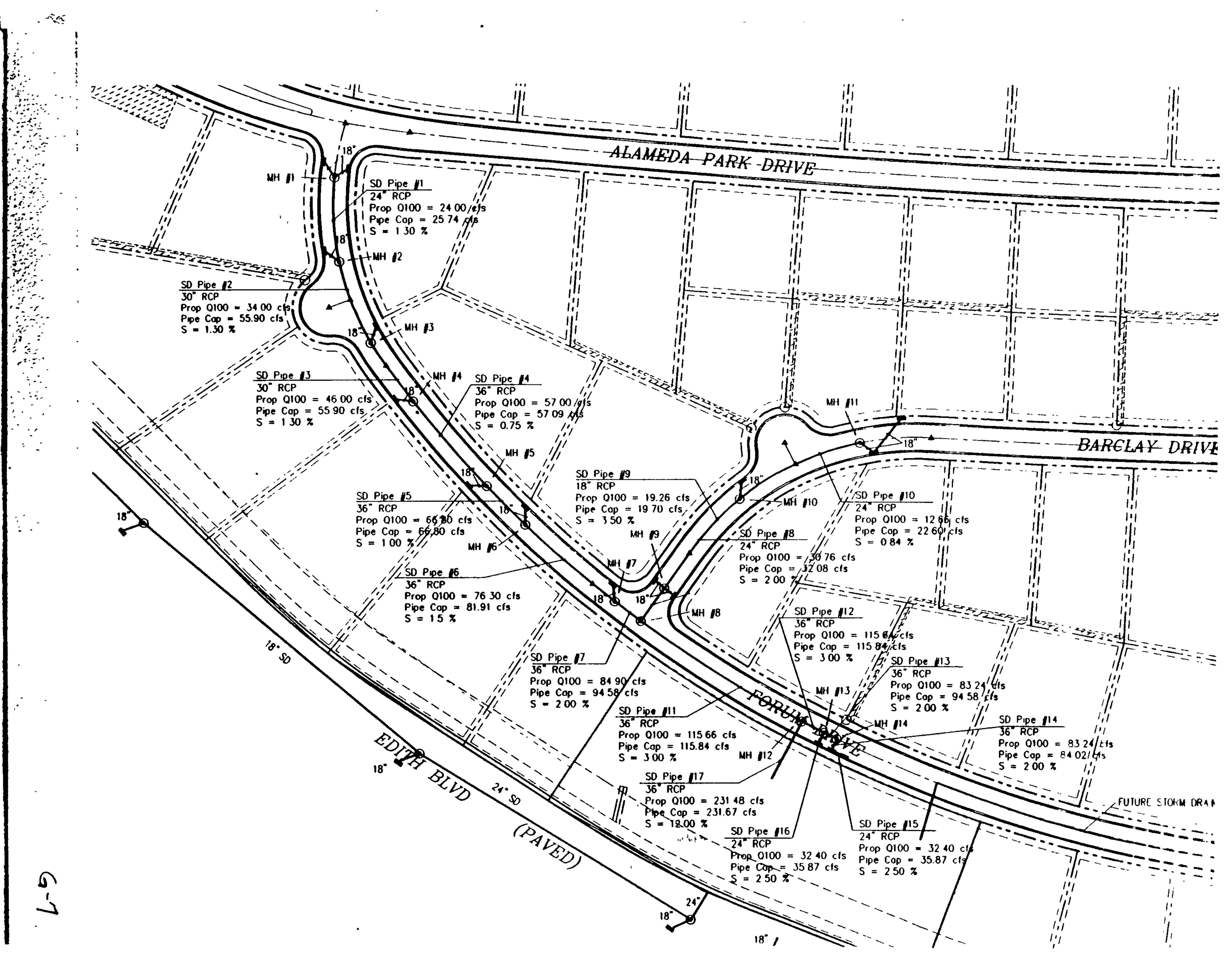
ANALYSIS OF AN INLET IN A SUMP CONDITION - EDITH BLVD EASTSIDE & WESTSIDE
