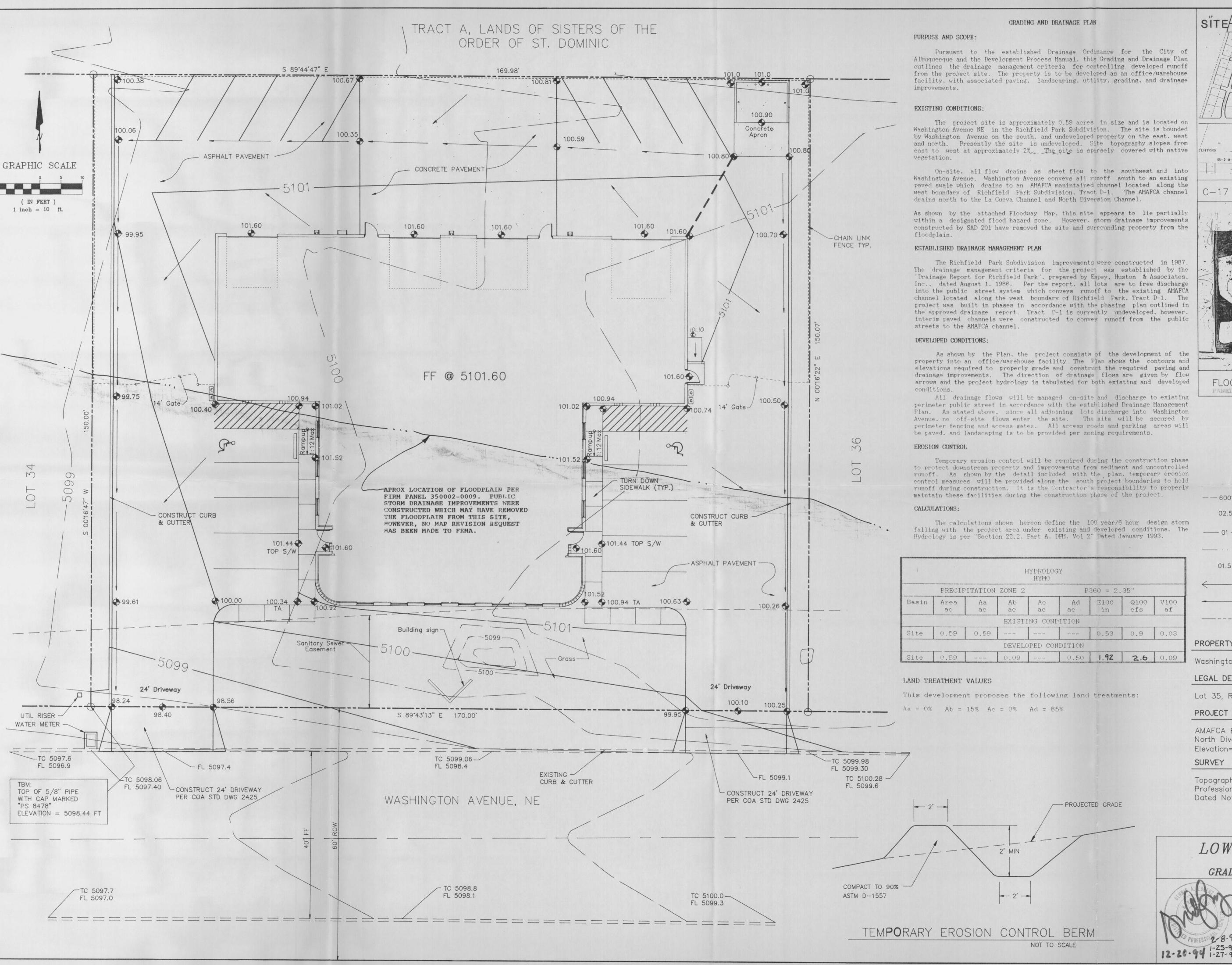
Albuquerque and the Development Process Manual, this Grading and Drainage Plan outlines the drainage management criteria for controlling developed runoff from the project site. The property is to be developed as an office/warehouse facility, with associated paving, landscaping, utility, grading, and drainage
