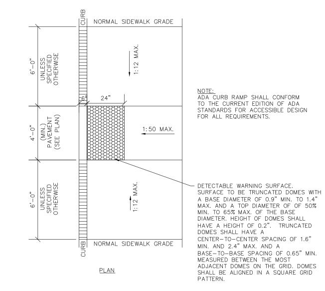
ADA SIDEWALK RAMP DETAIL NO SCALE
