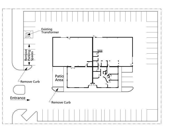
Floor Plan - Existing Reference Scale: 1" = 40'-0"
