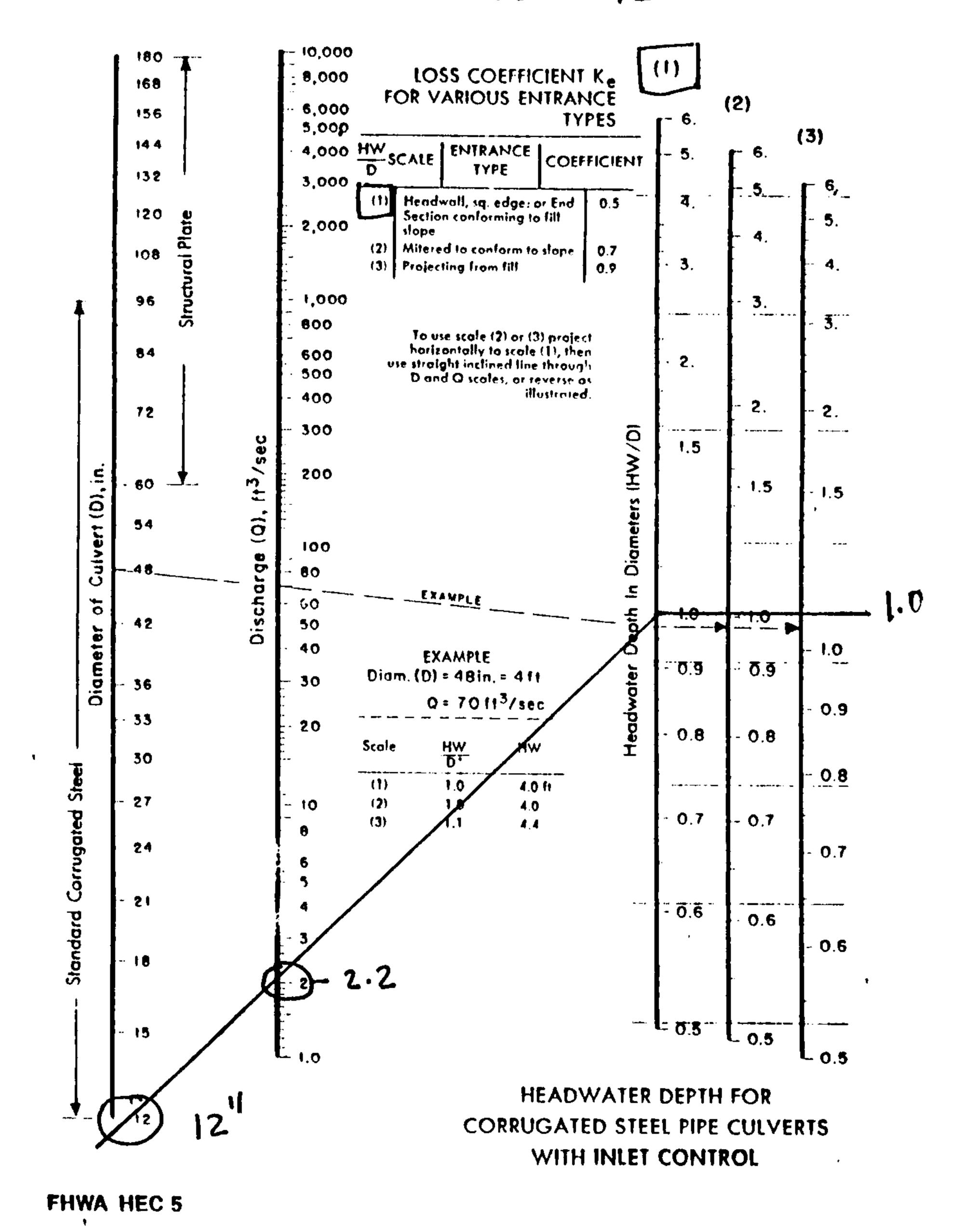
Figure 4-28 Inlet control nomograph for corrugated steel pipe culverts. The manufacturers recommended keeping HWID to a maximum of 1.5 and preferably to no more than 1.0.
