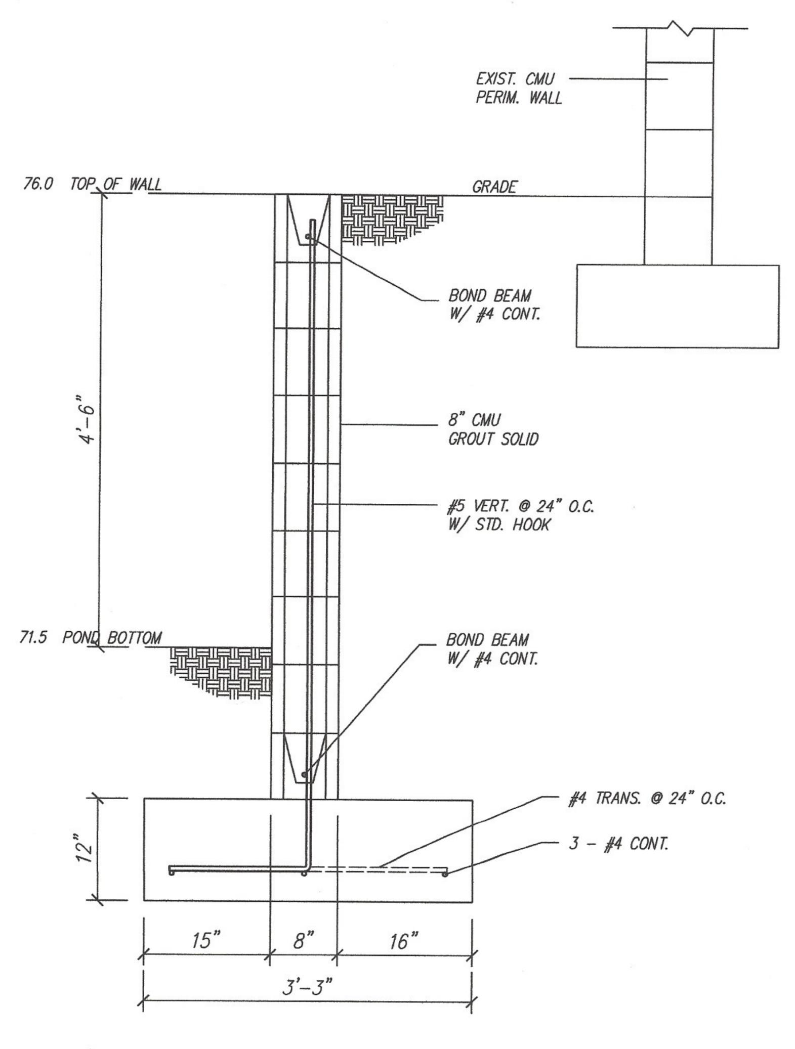
DETENTION POND RETAINING WALL SCALE: 3/4" = 1'-0"
