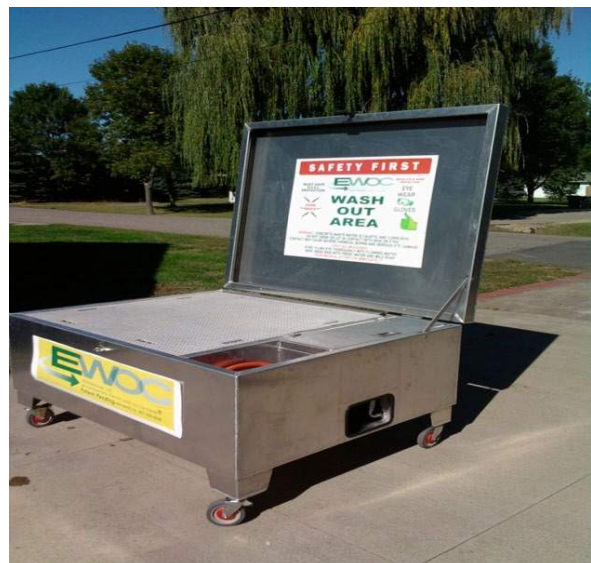
Self-contained washout facility
