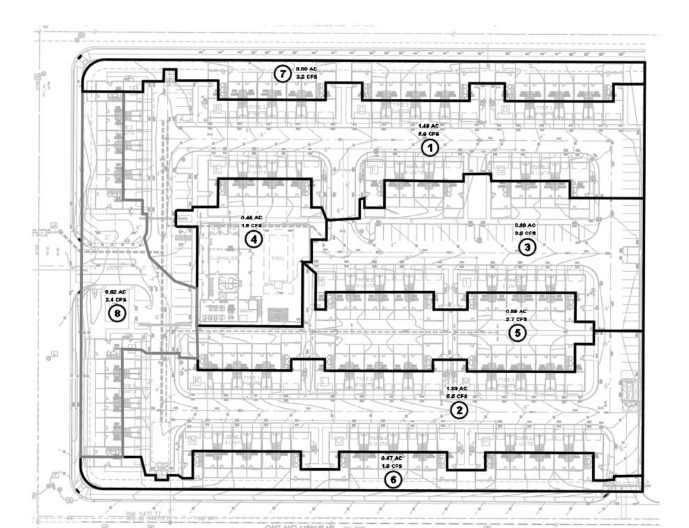
The conceptual drainage basin configuration shows Basins 6, 7 and 8 (approximately 6.2 cfs) being released to the adjacent streets. Stormwater quality ponds will be provided prior to the outfall as much as possible.
