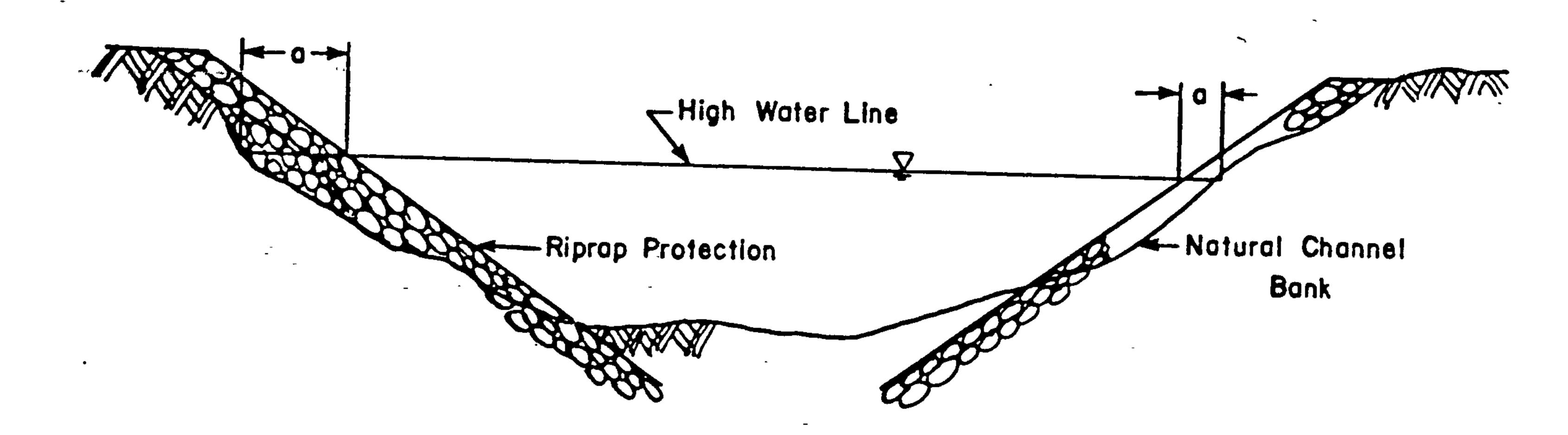
Figure 3-2. The embankment length measured normal to the flow.
