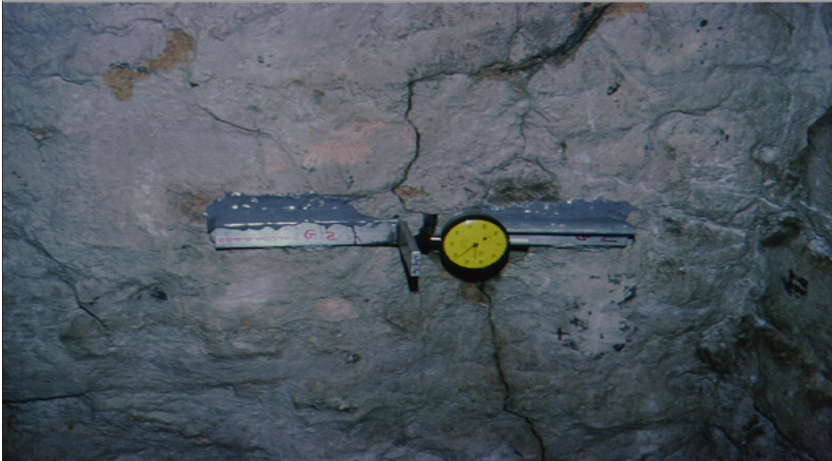
Figure 36.—Crack gage installed across a crack will allow determination of progressive widening or movement of the crack. It may be necessary to monitor such gages for periods up to a year to predict future crack behavior.
