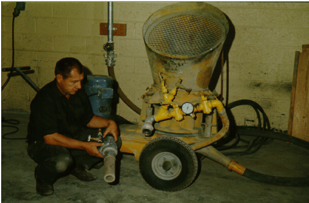
Figure 44.—Dry mix shotcrete equipment showing the nozzle and water injection ring.
