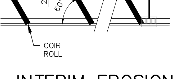
COIR ROLL DETAIL SCALE: 1"=2' WOOD STAKE COIR ROLL EXISTING SLOPE INBED COIR ROLL ±3" INTO EXISTING GROUND SURFACE TO PROVIDE CUTOFF
