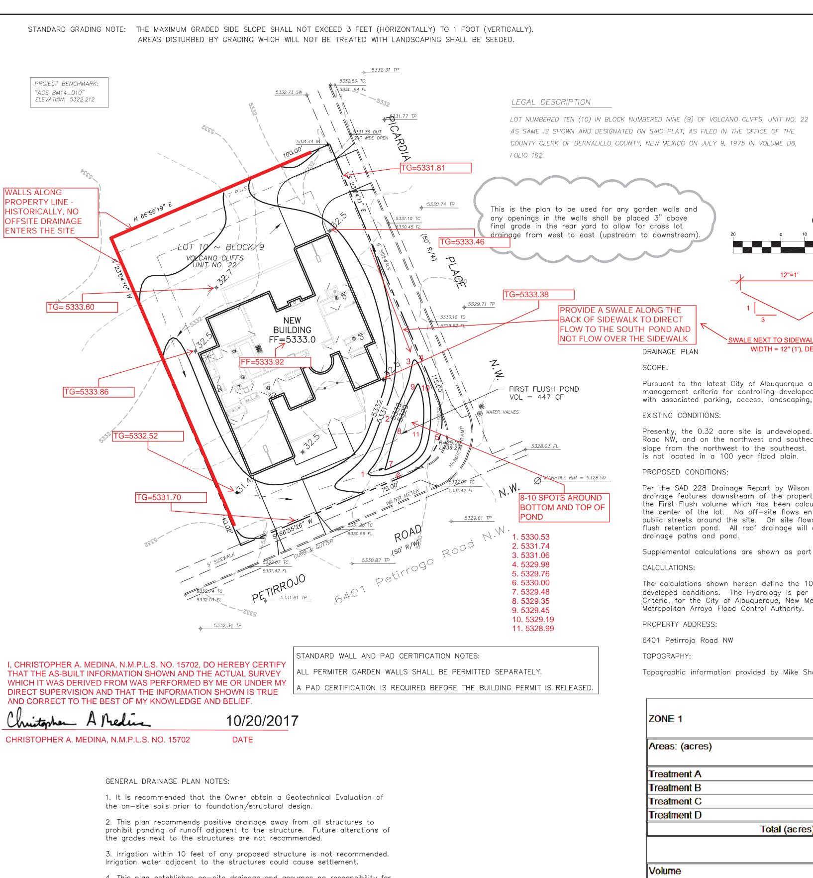
4. This plan establishes on—site drainage and assumes no responsibility for subsurface analysis, foundation or structural design, or utility design.
