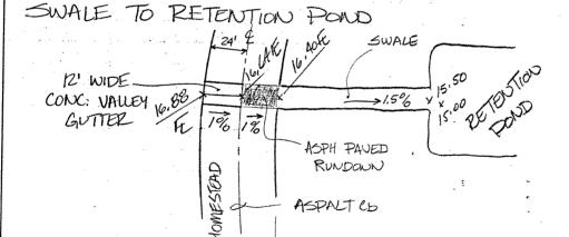
ASPHALT PAVED BUNDOWN (FIRST PORTION OF SWALE) Q100 = 28.4 CFS N= 0.016 (asph) 3=10/6 With D=12', Find depth of FLOW
