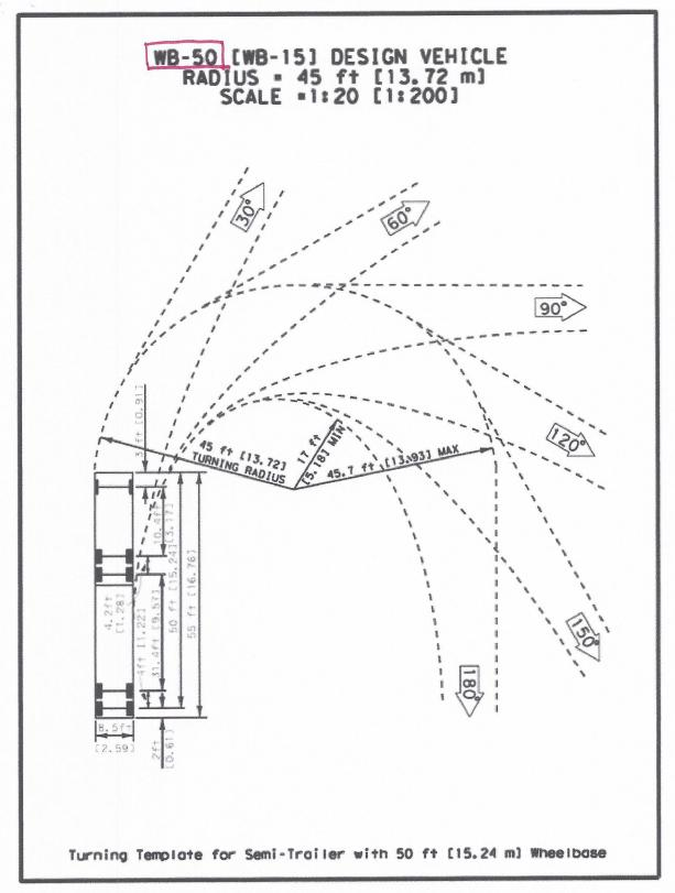
Figure 7-3. Turning Template for Semi-Trailer with 50 ft [15.24 m] Wheelbase, (not to scale).
