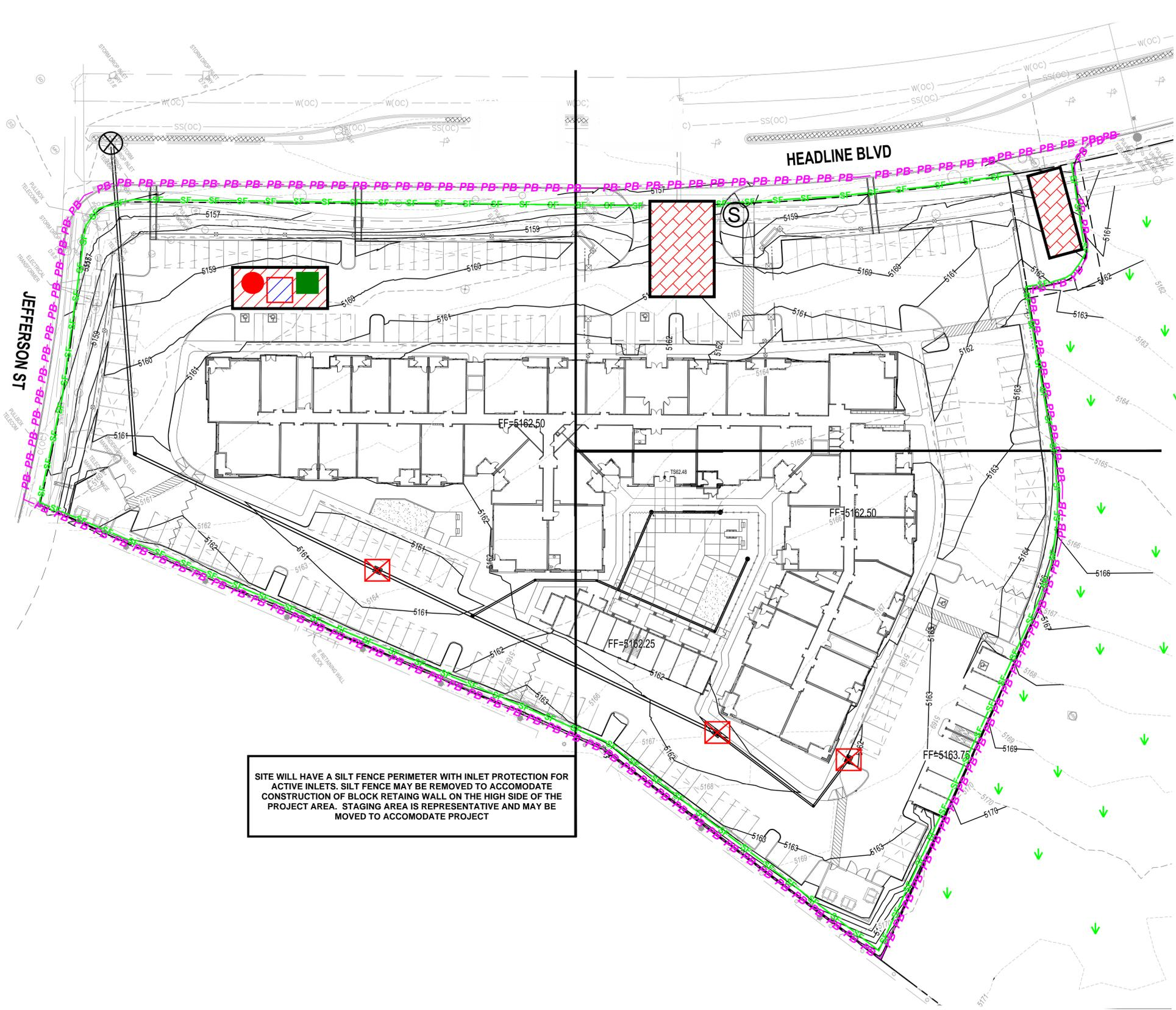
SITE WILL HAVE A SILT FENCE PERIMETER WITH INLET PROTECTION FOR ACTIVE INLETS. SILT FENCE MAY BE REMOVED TO ACCOMMODATE CONSTRUCTION OF BLOCK RETAINING WALL ON THE HIGH SIDE OF THE PROJECT AREA. STAGING AREA IS REPRESENTATIVE AND MAY BE MOVED TO ACCOMMODATE PROJECT
