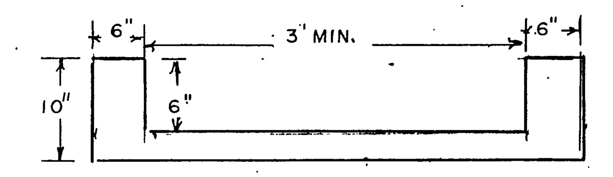
SECTION A---A PC CONCRETE OUTLET CHANNELS
