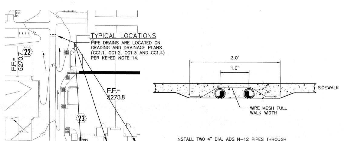
SIDEWALK. WHERE ADJACENT TO PAVEMENT, MATCH GUTTER FLOWLINE AT OUTLET. PROVIDE SWALE WITHIN
