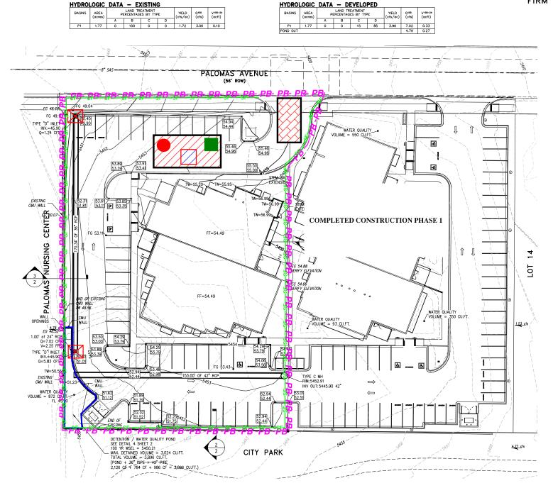
SITE WILL HAVE A PERIMETER SILT FENCE ATTACHED TO CHAIN LINK WITH A MULCH SOCK BASE. ALL DISTURBED AREAS SHAL BE STABILIZED PER THE CGP REQUIREMENT. STAGING AREA IS REPRESENTATIVE AND MAY BE MOVED TO ACCOMODATE PROJECT
