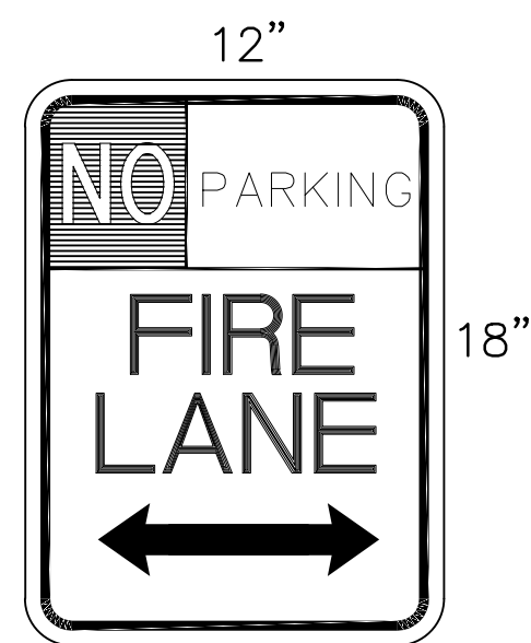
NO PARKING FIRE LANE SIGN
