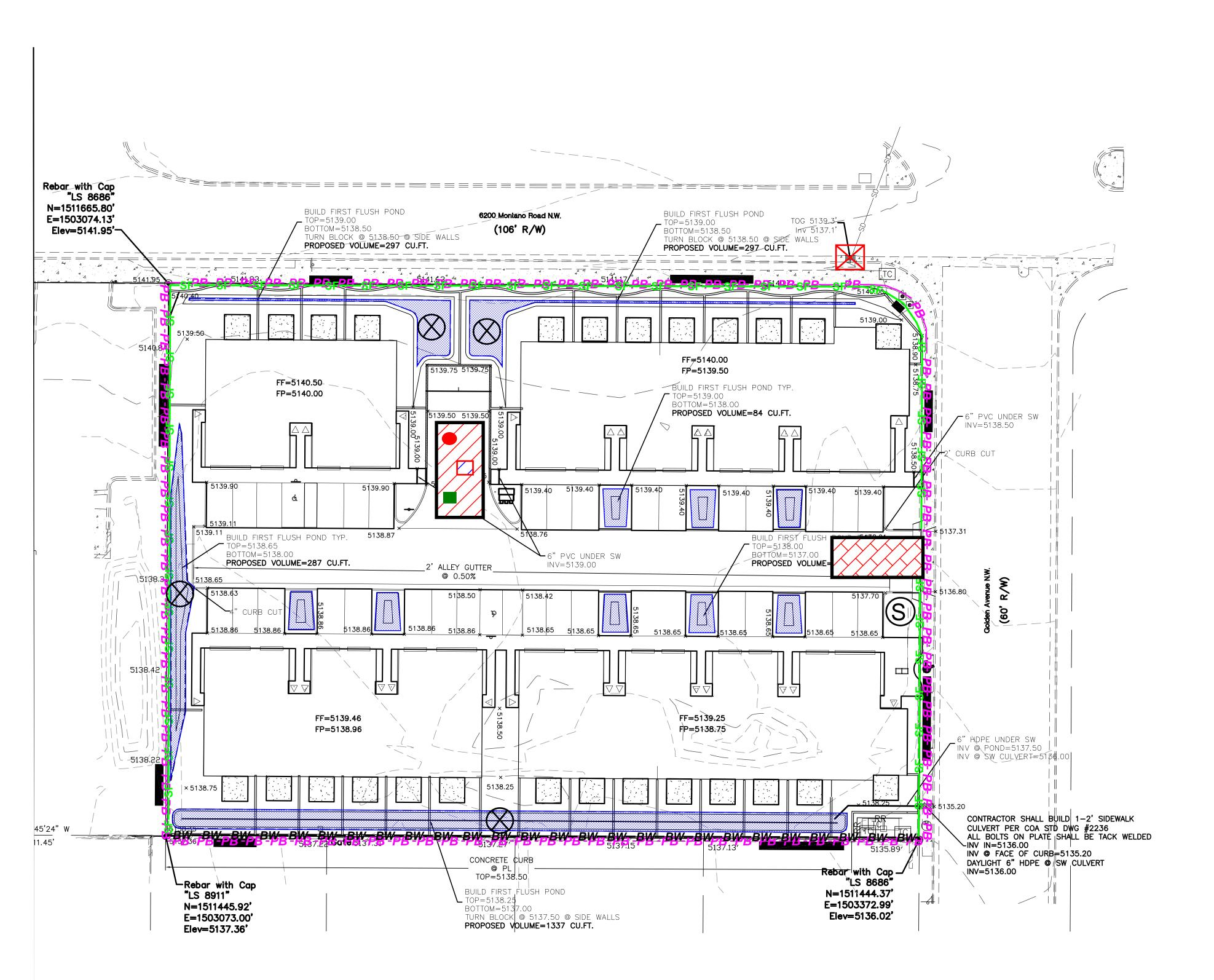
SITE WILL HAVE A SILT FENCE AND BLOCK WALL PERIMETER. FIRST FLUSH PONDS SHALL BE CONSTRUCTED DURING GRADING. STAGING AREA IS REPRESENTATIVE AND MAY BE MOVED TO ACCOMODATE PROJECT.
