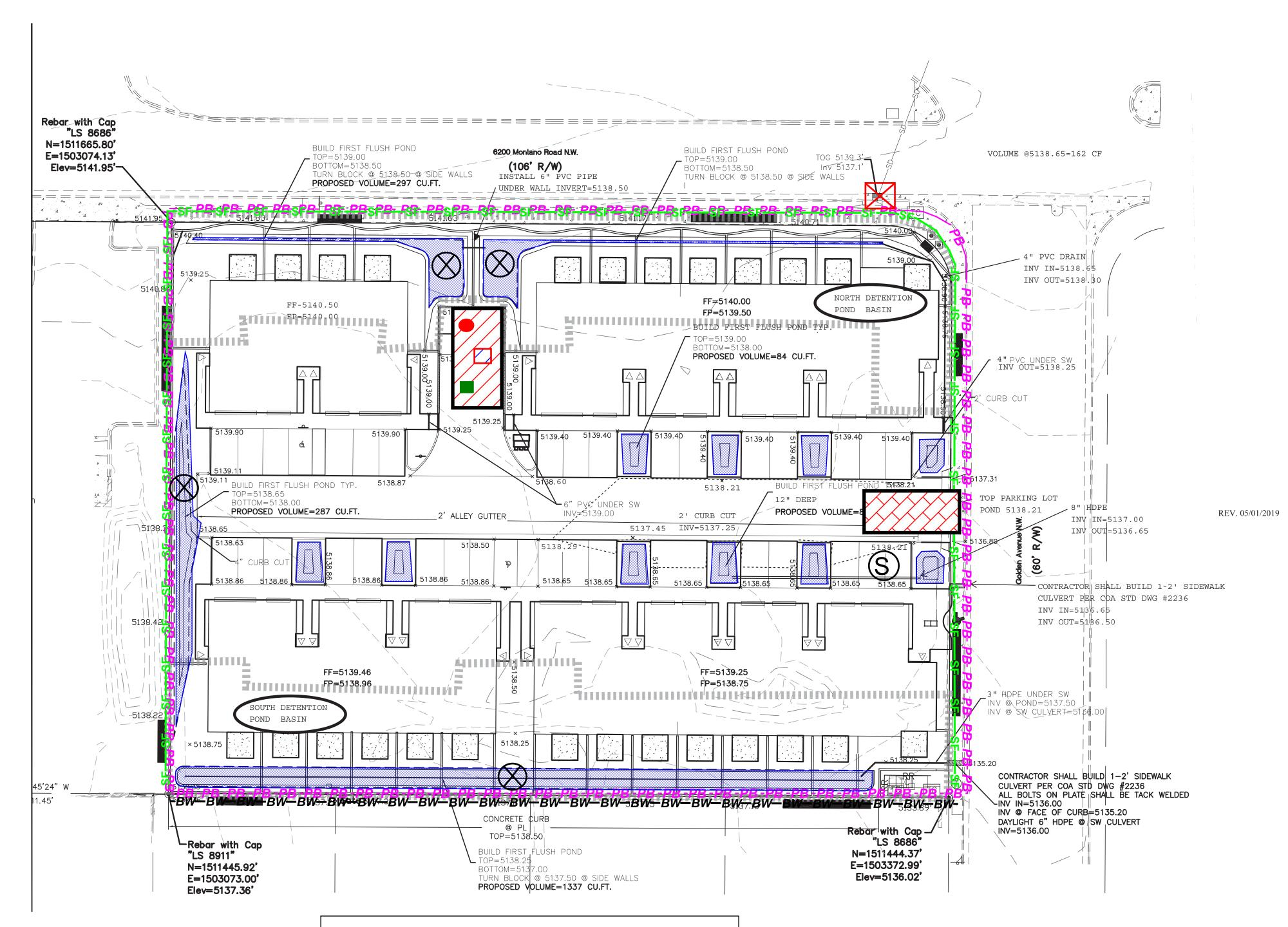
SITE WILL HAVE A SILT FENCE AND BLCK WALL PERIMETER. FIRST FLUSH PONDS SHALL BE CONSTRUCTED DURING GRADING. STAGING AREA IS REPRESENTATIVE AND MAY BE MOVED TO ACCOMODATE PROJECT.
