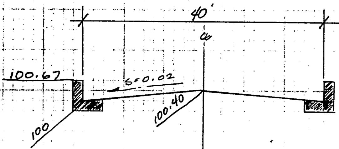
CAPACITY OF 1/2 STREET TO  $\phi$  (TOP OF CROWN)
