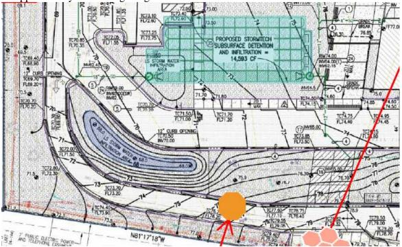
into the temporary pond at the time of inspection. Perhaps stormwater can infiltrate slowly through the top, but it is situated out of the flow path of surface drainage allowing a large portion of the site to bypass the pond.
