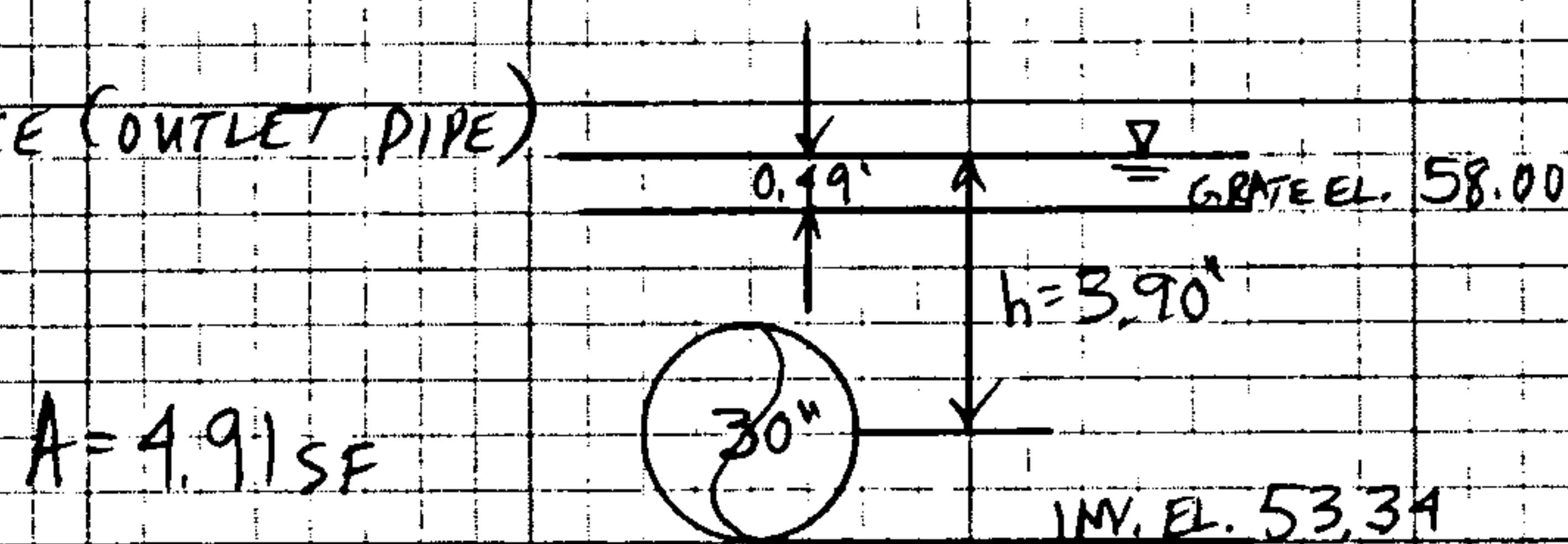
$$Q_{\text{CAP}} (\text{NO CLOGGING FACTOR}) = 46.7 \text{ cfs}$$
