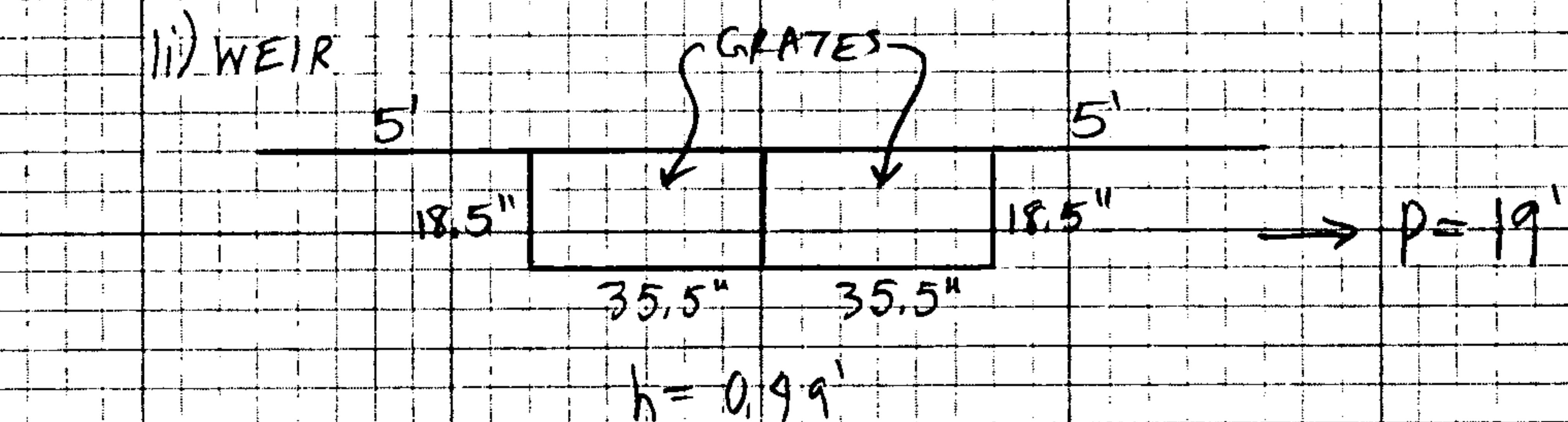
$$\text{CONTROLS} \rightarrow Q_{\text{CAP}} = 21.5 \text{ CFS}$$
