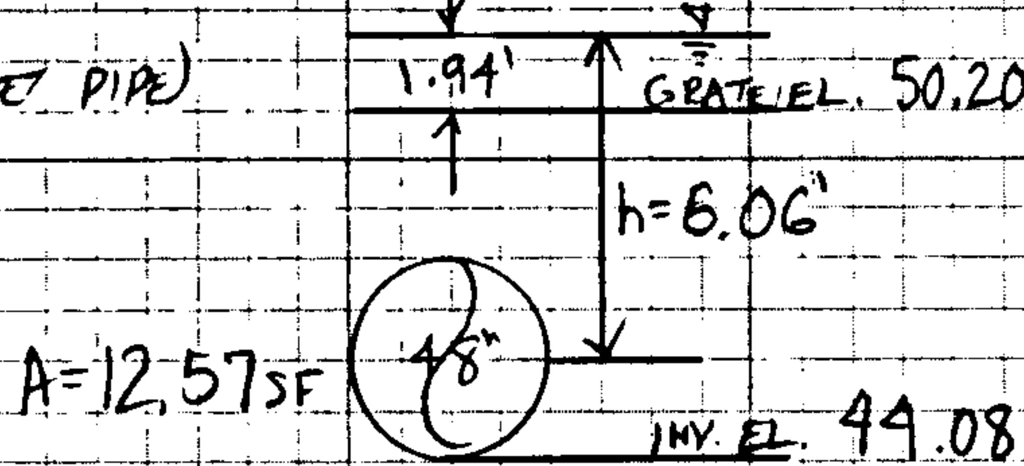
$$Q_{CAP} (\text{NO CLOGGING FACTOR}) = 149.0 \text{ cfs}$$
