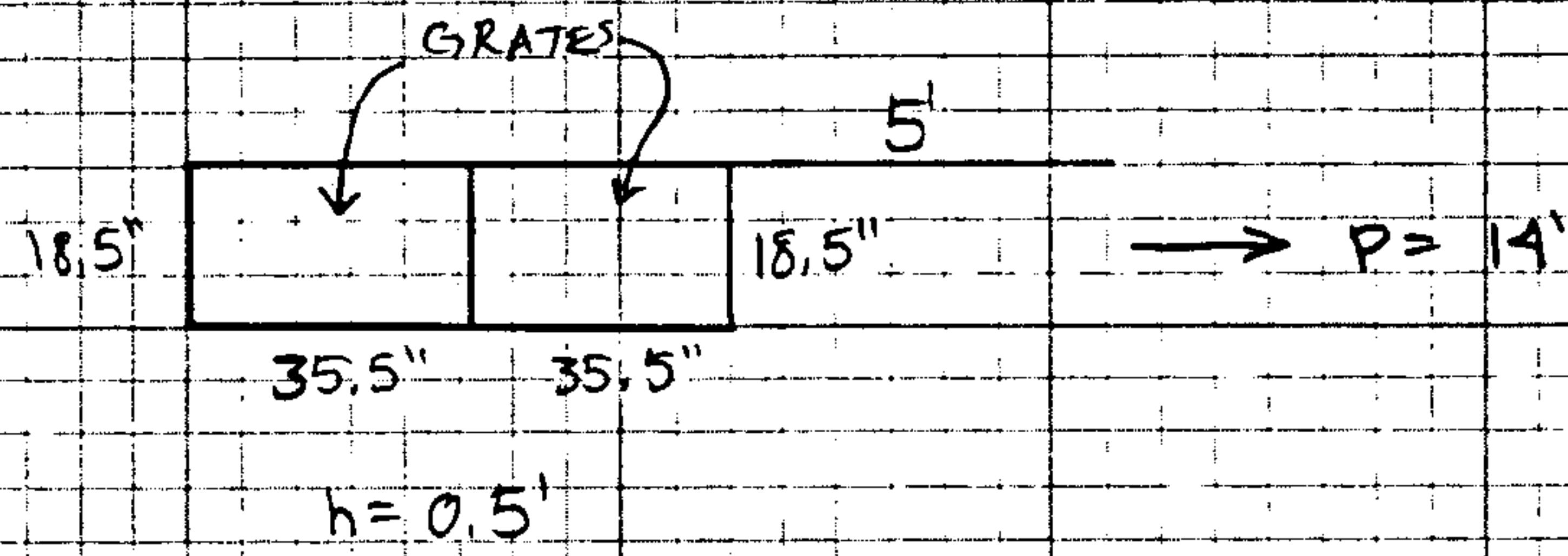
CONTROLS  $\rightarrow Q_{cap} = 11.4 \text{ cfs}$  INTO INLET
