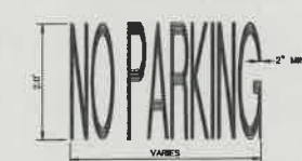
'No Parking' Striping Detail NTS
