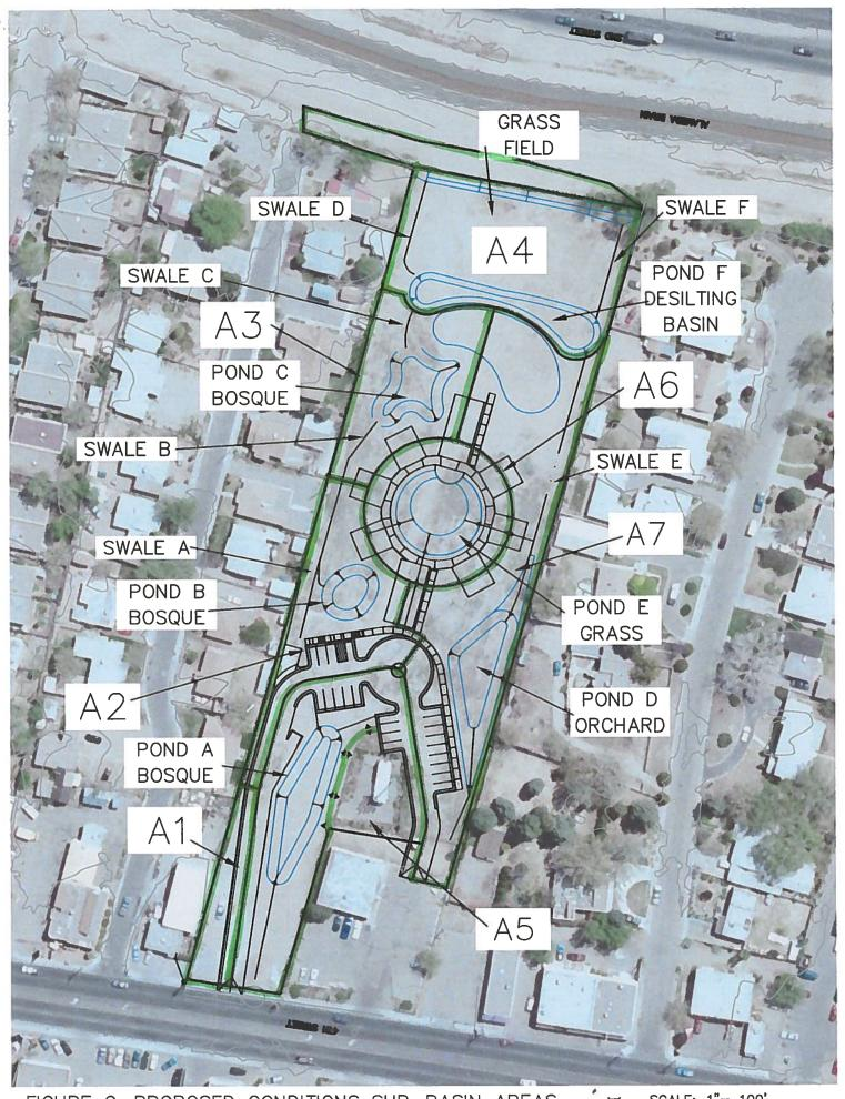
FIGURE C: PROPOSED CONDITIONS SUB-BASIN AREAS \_\_\_ SCALE: 1"= 100"
