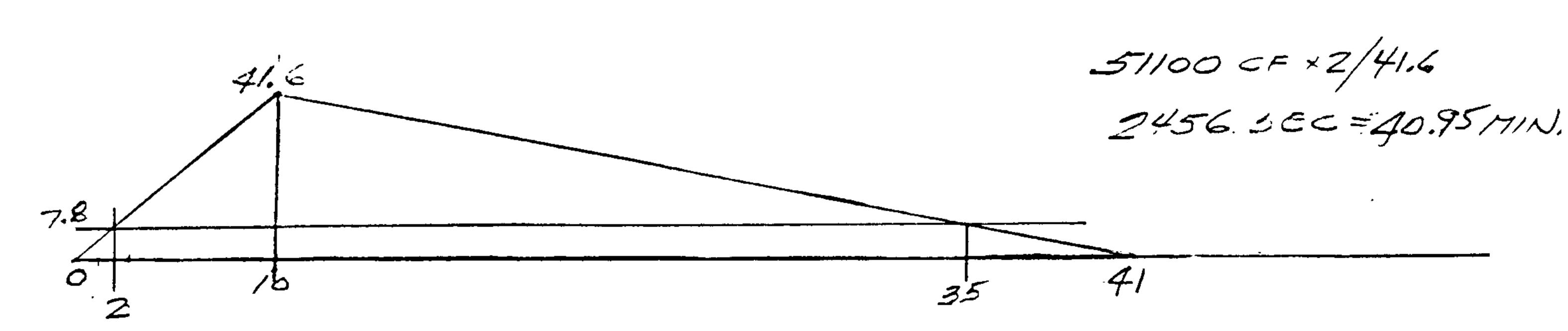
DISCHARGE VOLUME = 33 MIN. × 60 SEC. × 7.8 CFS = 15444 + 1.0 MIN × 60 SEC. × 7.8 CFS = 468 + 6.0 MIN × 60 SEC. × 7.8 CFS = 2808
