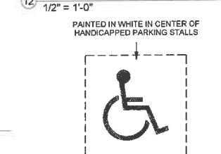
3 Accessible Parking Space Marking 1/4" = 1'-0"
