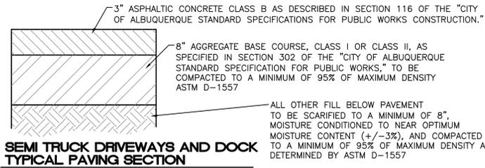
**SEMI TRUCK DRIVEWAYS AND DOCK TYPICAL PAVING SECTION**
