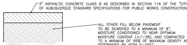
**AUTOMOBILE PARKING TYPICAL PAVING SECTION**
