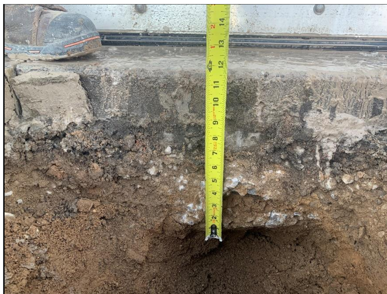
Test Pit (TP-3). Concrete thickness, approximately 12 inches
