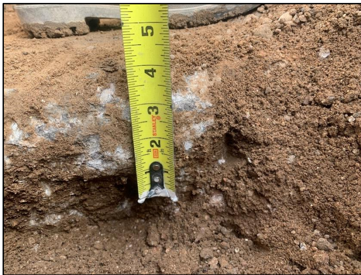
Test Pit (TP-2). Concrete thickness, approximately 4 ½ inches
