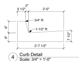
Per CoA std. dwg 2415A Provide 1/2" Expansion joints at 36" o.c. at immovable objects and at the beginning and end of curves
