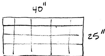
$$\begin{aligned} &\text{EFFECTIVE CLEAR OPENING} \\ &= 35.5'' \times 19.5'' \\ &= 692.25 \text{ SF} \end{aligned}$$
