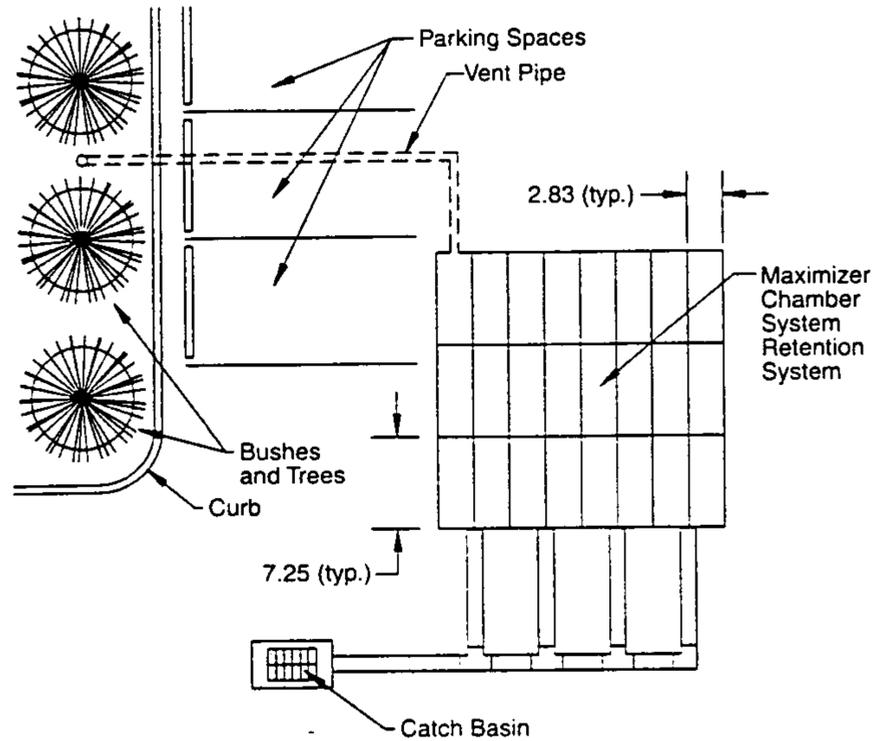
for every 500 square feet of bed area (or equivalent). Ventilation pipes must be outletted to "daylight" and protected from loading and accumulation of trash.
