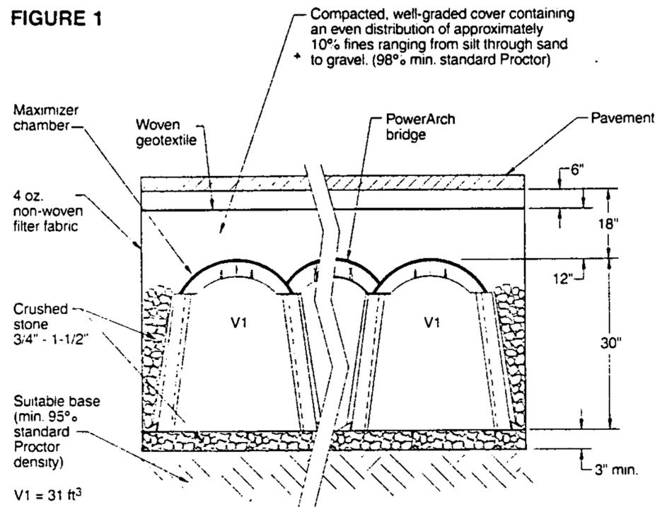
The PowerArch bridge spans the void between two chamber sidewalls. The top of the PowerArch bridge is arched and corrugated for structural strength. The nominal wall thickness of the PowerArch bridge is 0.15". Like the Maximizer chamber, the PowerArch bridge is equipped with interlocks that allow for the construction of rows of indefinite length. A 1.25" overlap is provided at the joints between the bridges. Two PowerArch bridges are needed to connect two parallel Maximizer chambers.
