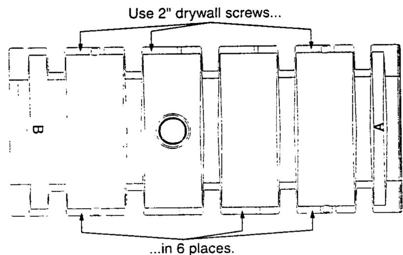
**10** Install the second bridge as the first, making sure that the "B" end lines up with the "B" chamber ends.
