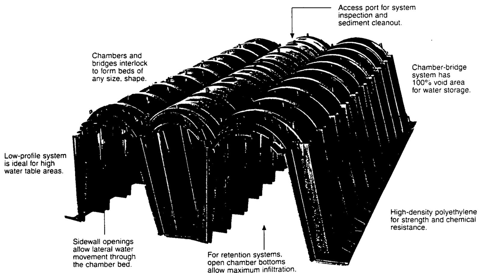
The Maximizer Chamber System is manufactured by Infiltrator Systems Inc. of Old Saybrook, Connecticut. The system is comprised of Maximizer chambers, PowerArch™ bridges, and endplates which fit the chamber ends and bridge ends, respectively. These structures are injection molded from high-density polyethylene. The density of the polyethylene is a minimum 0.950 grams/cubic centimeter (ASTM D1248, D1505).
