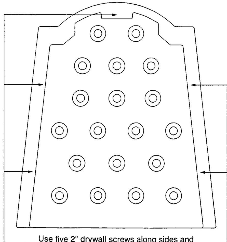
Use five 2" drywall screws along sides and top of the end plate to secure it to the chamber.
