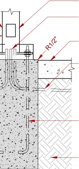
TWO-HEAD LIGHT POLE -SEE ELEC. DRAWINGS. **1" SEAL-TILE CONDUIT** FROM SECURITY EQUIP. LOCATION PREFERRED FINISH GRADE POSITION.
