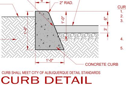
CURB NOTES: 1. CONCRETE TO BE 3000 PSI MINIMUM. DUMMY JOINT REQUIRED AT 10' O.C. SEALED EXPANSION JOINTREQUIRED AT CURB RETURNS WITH 1/2" PREMOLDED ASPHALT IMPREGNATED EXPANSION MATERIAL OR EQUAL. **EXPANSION JOINTS REQUIRED AT 50'** O.C. WHEN FORMING FOR CURBS. PROVIDE EXPANSION JOINT MATERIAL WHERE SIDEWALK MEETS CURB, AND AT ALL SIDES WHERE CONCRETE
