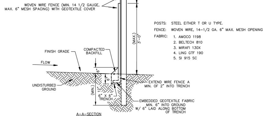
1. WOVEN WIRE FENCE TO BE FASTENED SECURELY TO FENCE POSTS WITH WIRE TIES.
