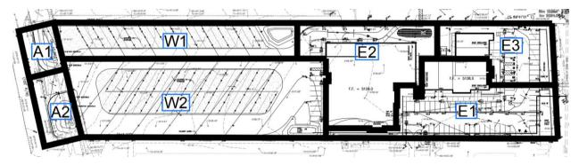
The portion of Atrisco Road along the property frontage will be ponded within the adjacent R.O.W. The ponds will be constructed to retain the 100-year 10-day storm event. As noted on the plan, no work shall be performed in the public row without an approved work order or excavation permit.
