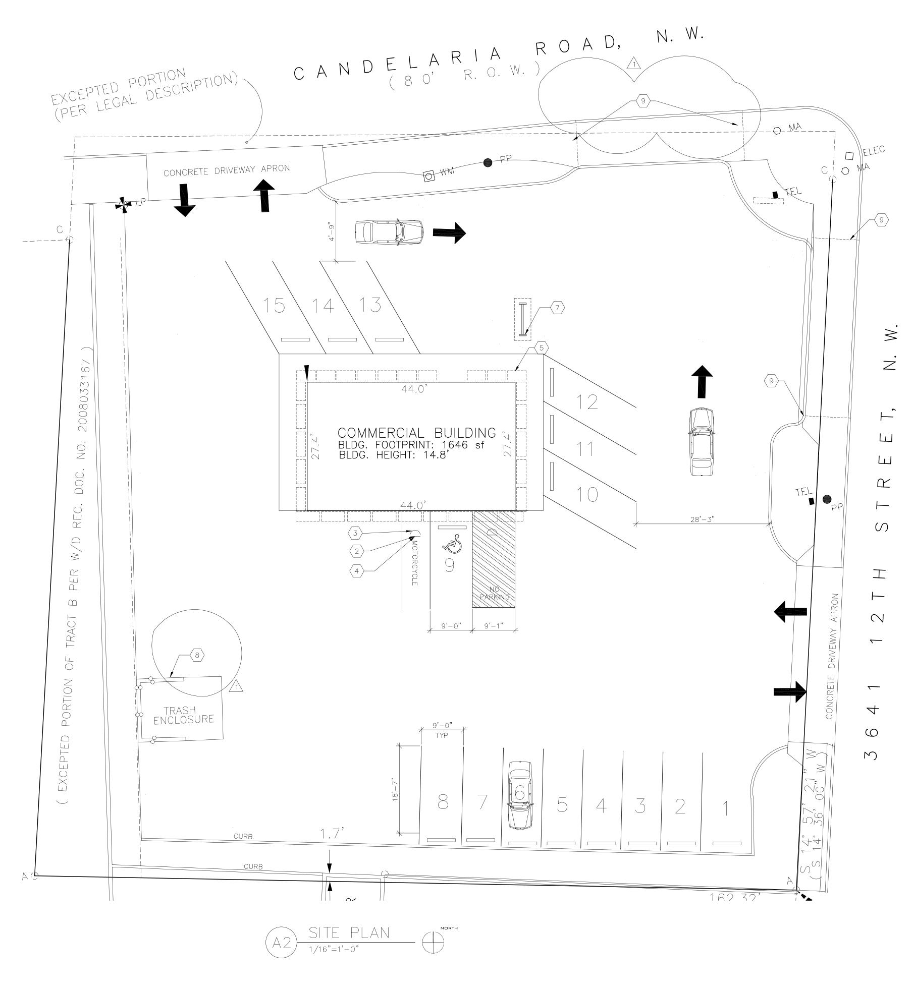
NOTE 1: EXISTING LANDSCAPE AND SIGNAGE TO REMAIN. ALL NEW LANDSCAPING AND SIGNAGE WILL NOT INTERFERE WITH CLEAR SIGHT REQUIREMENTS. THEREFORE, SIGNS, WALLS, TREES, AND SHRUBBERY BETWEEN 3 AND 8 FEET TALL (AS MEASURED FROM THE GUTTER PAN) WILL NOT BE ACCEPTABLE IN THE CLEAR SIGHT TRIANGLE.
