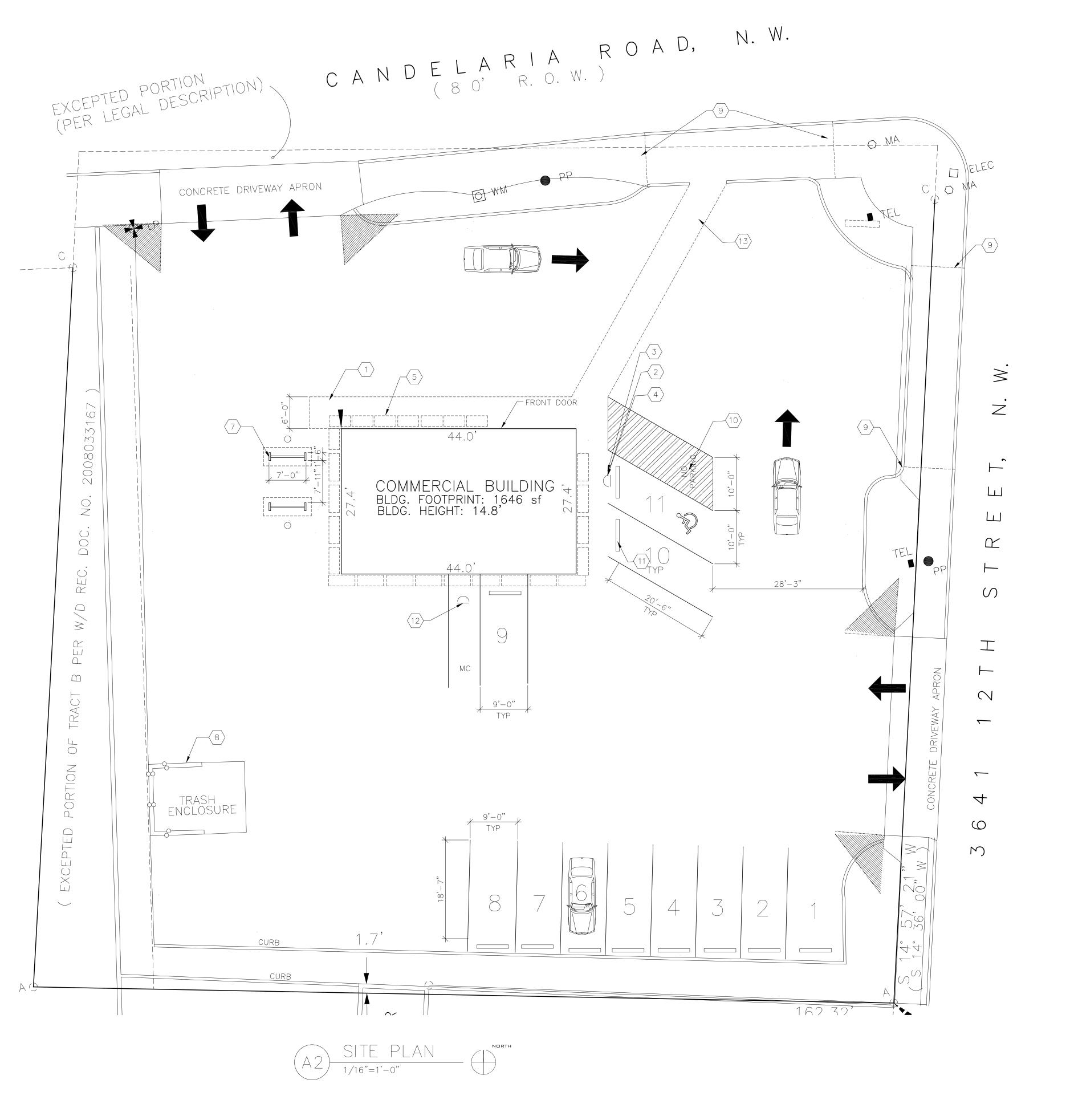
NOTE 1: EXISTING LANDSCAPE AND SIGNAGE TO REMAIN. ALL NEW LANDSCAPING AND SIGNAGE WILL NOT INTERFERE WITH CLEAR SIGHT REQUIREMENTS. THEREFORE, SIGNS, WALLS, TREES, AND SHRUBBERY BETWEEN 3 AND 8 FEET TALL (AS MEASURED FROM THE GUTTER PAN) WILL NOT BE ACCEPTABLE IN THE CLEAR SIGHT TRIANGLE. NOTE 2:N/A
