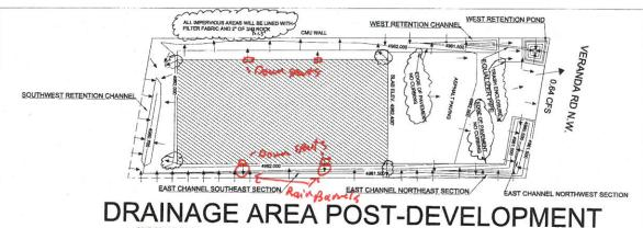
**ROOF WATER IS** HARVESTED ON-SITE FROM THE 4 DOWNSPOUTS TO THE CHANNELS
