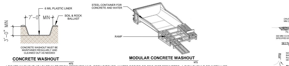
LOCATE WASHOUT AT LEAST 50 FT FROM STORMDRAINS, OPEN DITCHES, WATER BODIES OR PROJECT PERIMETER. A SIGN SHOULD BE INSTALLED ADJACENTLY TO THE WASHOUT.
