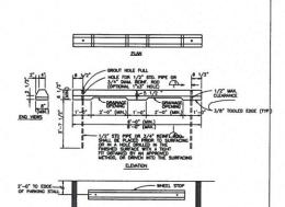
Precast Concrete Wheel Stop NTS
