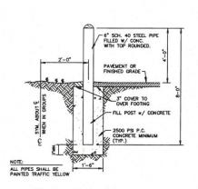
6" Pipe Bollard Detail NTS
