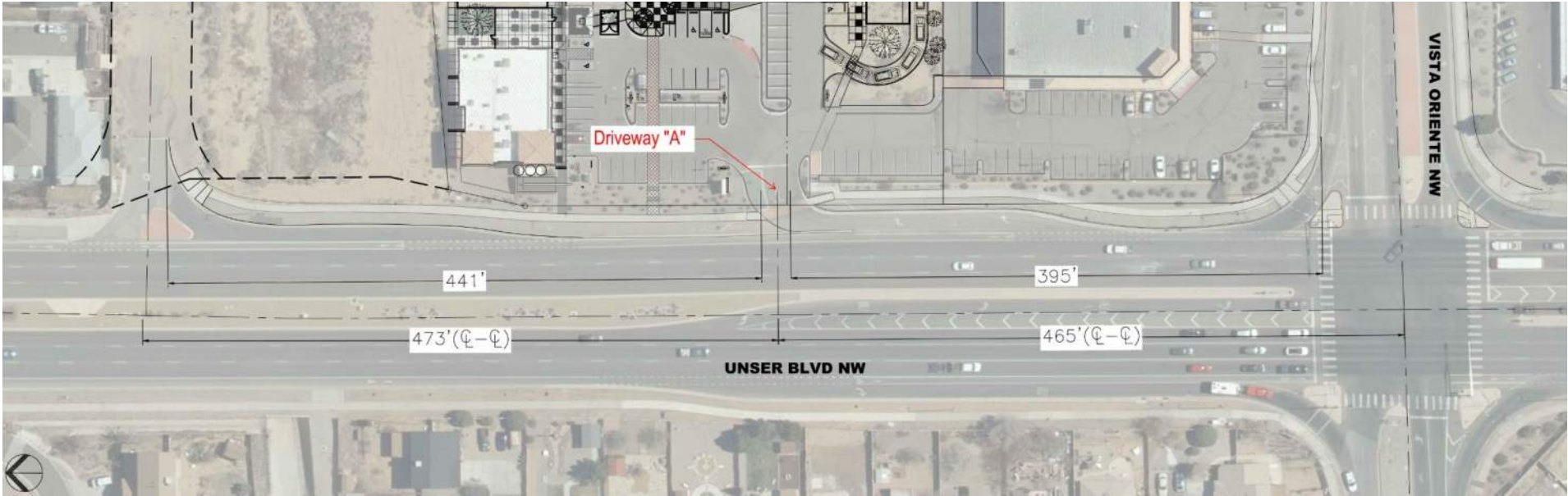
Figure 23 - Access Spacing: Driveway "A"
